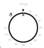
**NOTE:** For any time below fifteen minutes turn the knob past the fifteen then turn it back to the required number of minutes. When the timer returns to zero, the timer gives a short ring.
