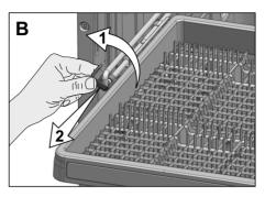
After taking out the basket by lifting it up, remove the carrier part from the rails by pulling it towards yourself (C).
