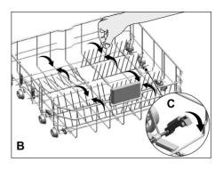
Bringing the tines to the horizontal position by holding them from the tips may cause them to bend. Therefore, it will be appropriate to bring the tines in the middle to horizontal or vertical position by holding them from their stems and pushing in the direction of arrow.
