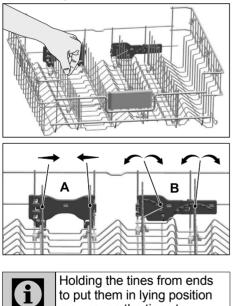
Holding the tines from ends to put them in lying position may cause the tines to bend. For this reason, it will be appropriate to hold the tines in the middle from their bottoms and to push in the direction of the arrow to lay down or bring them to vertical position.
