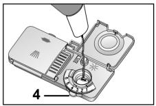
Turn the rinse aid amount adjuster manually to a position between 1 and 6 (4). If there are stains on tableware items after washing, level must be increased and if there is a blue trace after wiping them by hand, it must be decreased. This is
