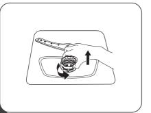
1 Hold the coarse filter and rotate it counter-clockwise to unlock the filter. Lift the filter upwards and out of the dishwasher.
