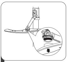
To remove the upper spray arm, hold the nut, rotate the arm clockwise to remove it.
