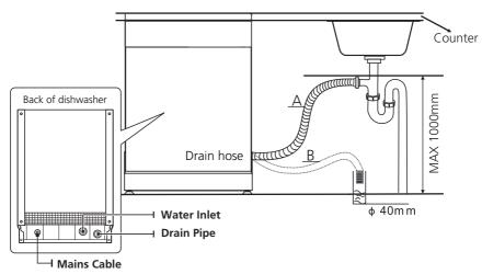
A Please securely fix the drain hose in either position A or position B
