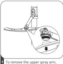
To remove the upper spray arm hold the nut, rotate the arm clockwise to remove it.
