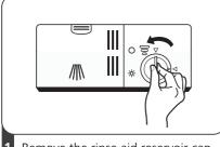
Remove the rinse aid reservoir cap by rotating it counter-clockwise.
