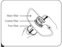
The fine filter can be pulled off the bottom of the filter assembly. The coarse filter can be detached from the main filter by gently squeezing the tabs at the top and pulling it away.
