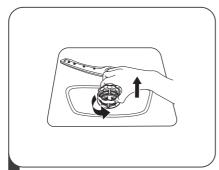
Hold the coarse filter and rotate it anti clockwise to unlock the filter. Lift the filter upwards and out of the dishwasher.
