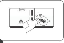
2 Carefully pour the rinse-aid into its dispenser, whilst avoiding any overflow.
